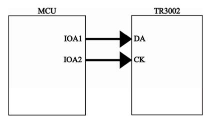
(6). The program example below is the code for the 4 bit MCU (tenx technology inc.) to control TR3002 and lock the 87.5MHz [445C(hex)] signal (transmit the CK and DA signal via IOA port, and define IOA2=CK, IOA1=DA)
